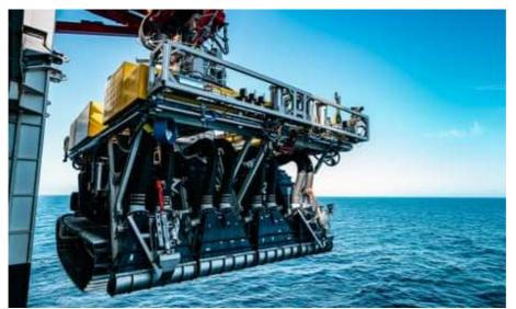
A pilot vehicle – called a nodule collector – used in deep-sea exploration is lowered into the water in trials conducted by mining group TMC. Photograph: Richard Baron/The Metals Company
