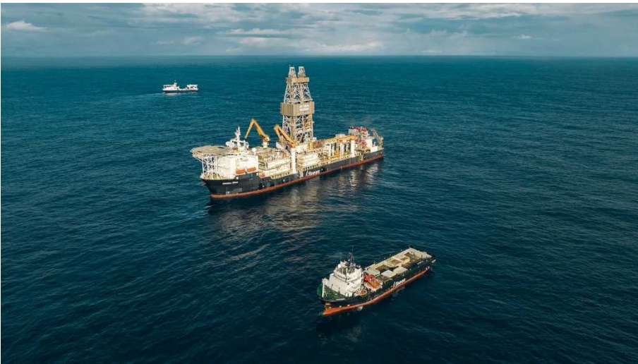
The Metals Company uses a former oil-drilling vessel, the Hidden Gem , to collect polymetallic nodules from the seafloor. Courtesy of Richard Barron/TMC
