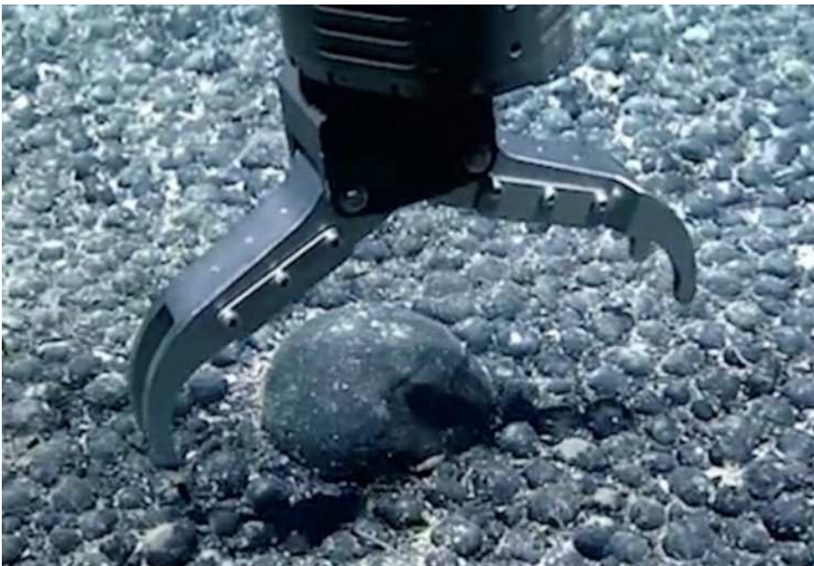
A polymetallic nodule is captured on a seamount deep in the North Atlantic Ocean during the 2021 North Atlantic Stepping Stones expedition. Credit: U.S. Geological Survey and NOAA Ocean Exploration.
