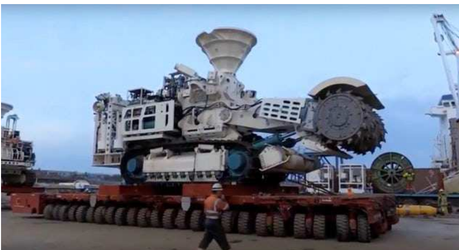
A seabed mining machine built for Nautilus Minerals. YouTube/Nautilus Minerals
